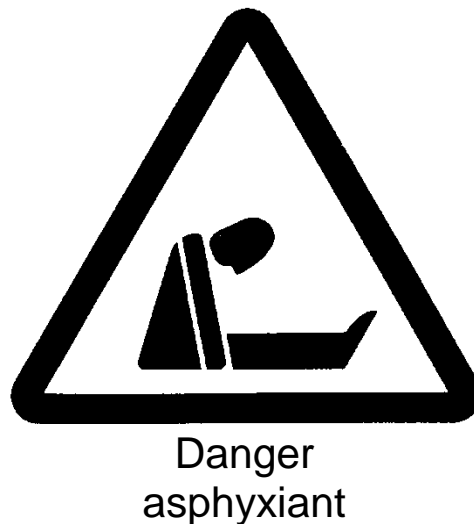
Fig.1 Asphyxiation hazard warning sign
