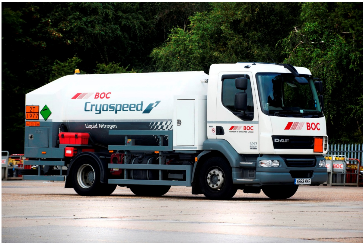
Fig.4 Typical cryogenic road tanker (courtesy BOC)
